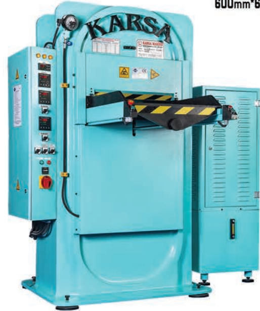
SAYA PRESİ (SHOE-UPPER PRESS) KM-415 405 TON 300 BAR 600mm*600mm
